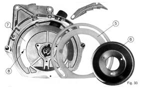
On the outside of the main housing is the lever for adjusting the air suction to the weight of the seed, as well as setting the height of the seed scraper.
