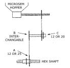
**A** = Double sprocket on hex shaft - driven 1 **B** = Interchangeable sprocket - driven 2
