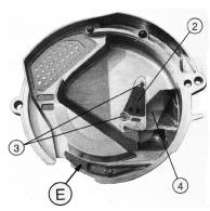
2– **Low Position:** For small seeds, such as cucumbers, beet, peppers, etc. The low position moves the shutter over part of the opening.
