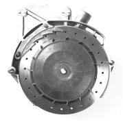
The stationary part of the metering box is called the main housing. shown below. and is mounted in the planter unit frame.
