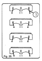
The drive is normally mounted in the center of the machine, as close as possible to the left side of the gearbox. For narrow inter-row spacing this drive can be placed on the outside of the toolbar frame. In that case, an optional bearing (#4515) can be used.
