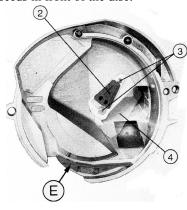
1 – **High Position**: **For large seeds**, such as corn, soybean, edible beans, cotton, etc. The high position moves the shutter away from the opening.
