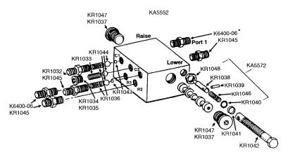
The valve block assembly consists of the marker sequencing and flow control valves in one assembly. The sequencing valve consists of a chambered body containing a spool and series of check valves to direct hydraulic oil flow. Should the valve malfunction, the components may be removed for inspection as follows:
