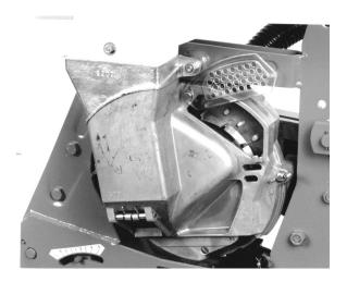
The metal shutter regulates the flow of seeds coming from the hopper and provides a constant and sufficient level in front of the disc. According to the seed used, the shutter has to be checked and adjusted at 2 different positions before planting.
